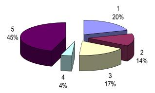
Figure 2. Failures, according to the environment, highlighted by HALT [7]. (1) Fast vibration thermal transitions with 6 degrees of freedom. (2) Extreme low temperature. (3) Extreme high temperature. (4) Fast thermal transactions. (5) Vibration with 6 degrees of freedom.
