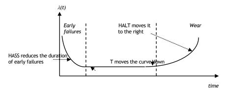
Figure 5. Influence of HALT and HASS on the bathtub curve [9]
