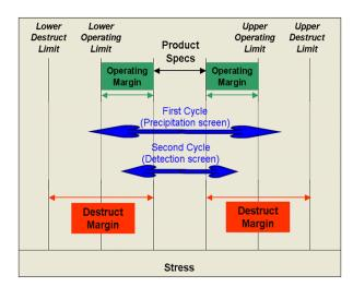
Figure 4. HALT stress thresholds
