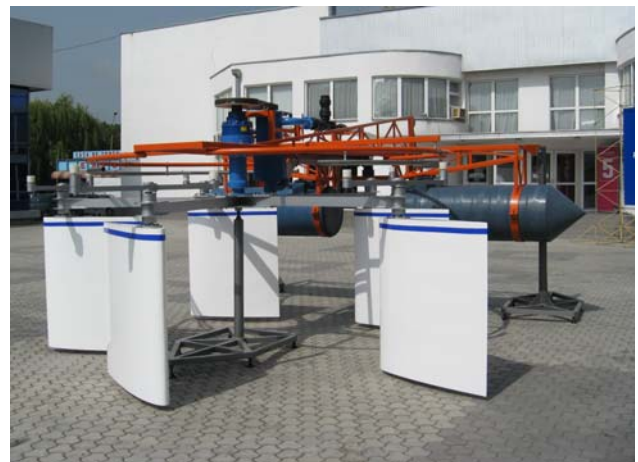
Figure 5. Industrial prototype of micro-hydro power plant river water kinetic energy conversion.
