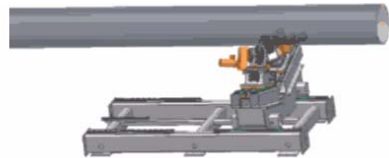
Fig. 5. Simulation of the both sides welding process (By courtesy of PWS GmbH)
