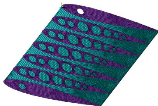
Figure 3: Discretization of the blade lateral cover into finite elements.
