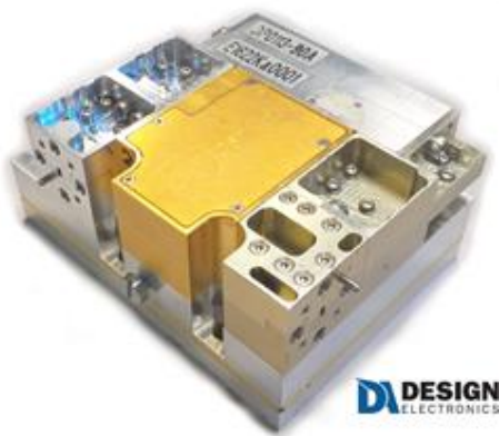
Fig. 2 89 GHz detector module (centre) implemented into the 89 GHz breadboard receiver by DA Design.
