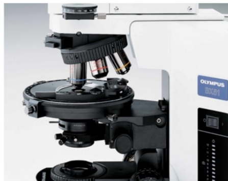
Fig.2. Microscop optic model Olympus BX 51 [18].
