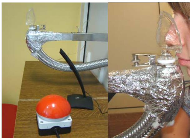
Figure 2. Sniffing-port (with the glass mold of the nose), button and microphone for recording.
