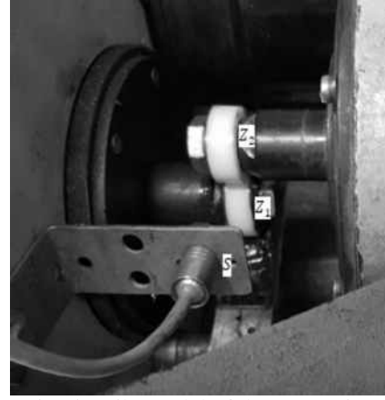
Fig. 5. Tribomodel of the precessional gear: Z_1 - model roller of immobile central wheel teeth; Z_2 - model roller of satellite wheel teeth; S - digital infrared pyrometric sensor for temperature measurement (model Impac IN 150)
