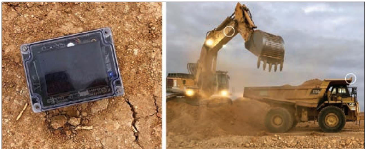
Figure 2. Smart nodes and their location on the machines [2]
