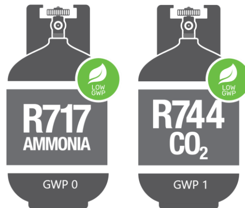
Figure 3. Low GWP refrigerants
