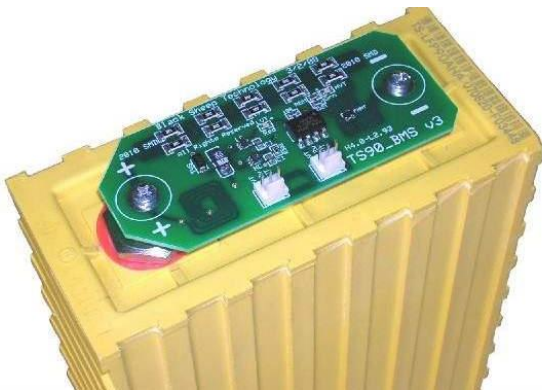
Fig. 5. Battery monitoring system (BMS).
