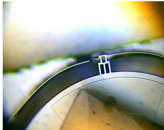
Figure 4. Construction damage occurred during assembly and drying processes.
