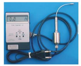
For convenient use of the device in both laboratory conditions and less equipped devices, it possesses low power consumption provided by a power supply unit of 220V AC or 9V battery power, indicated by a green LED. Red LED generates a warning signal, indicating low battery voltage, below 7V, because the microcontroller needs minimum stabilized 5V power. Error measurements occur guaranteed at further galvanic element discharge.
