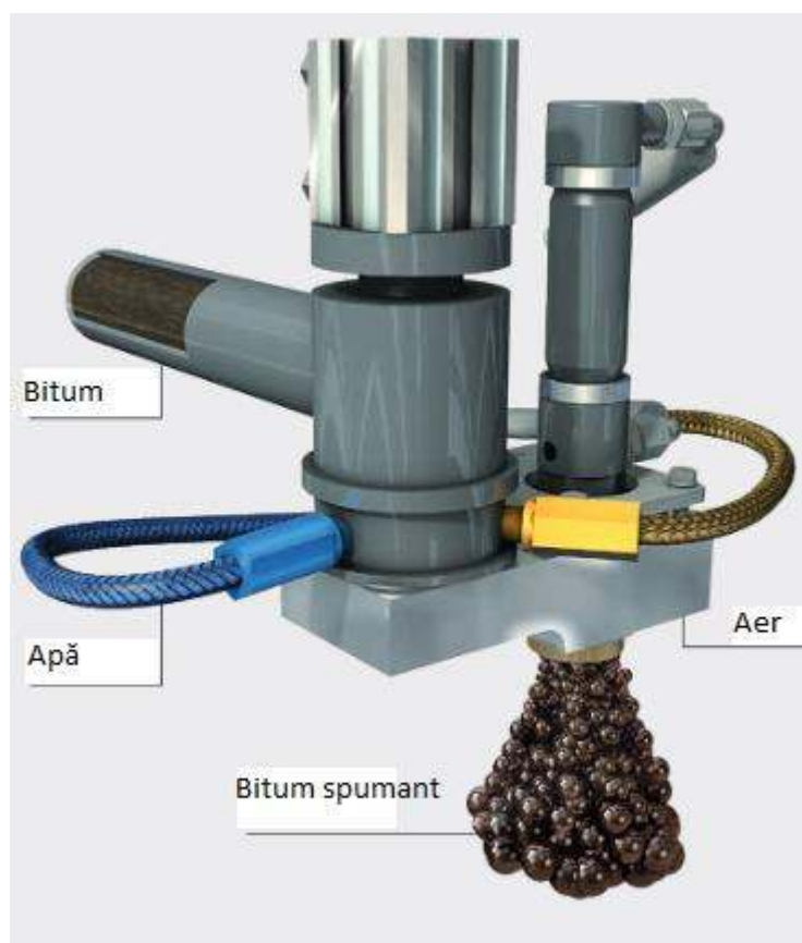
Figura 1. Producerea spumei de bitum
