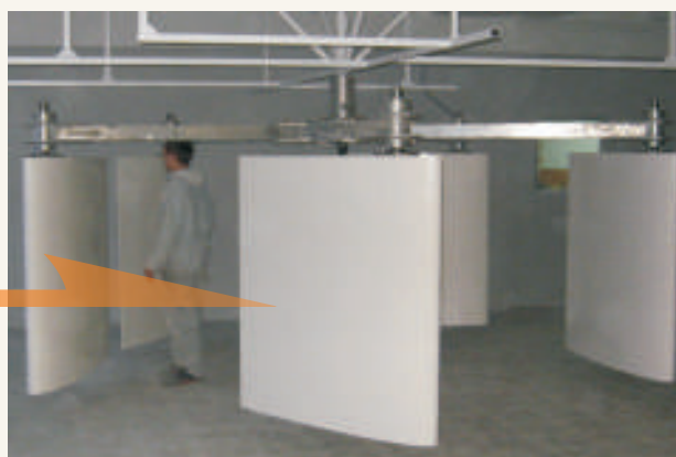
f) Assembled 5-blade hydrodynamic rotor.
