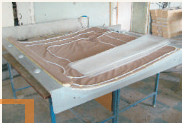
b) Installation of membrane and vacuum accessories into the form.
