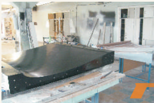
a) Manufacture of NACA profile form 0016 invertat.
