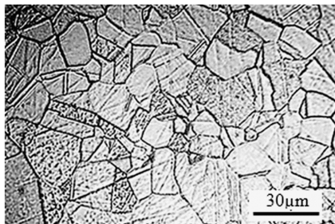
Figure 1. Microstructure image of surface of AISI 316L austenitic stainless steel after chemical etching.
