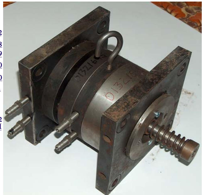
Figure 2. Mold of plastic gear wheels in the precessional gear.
