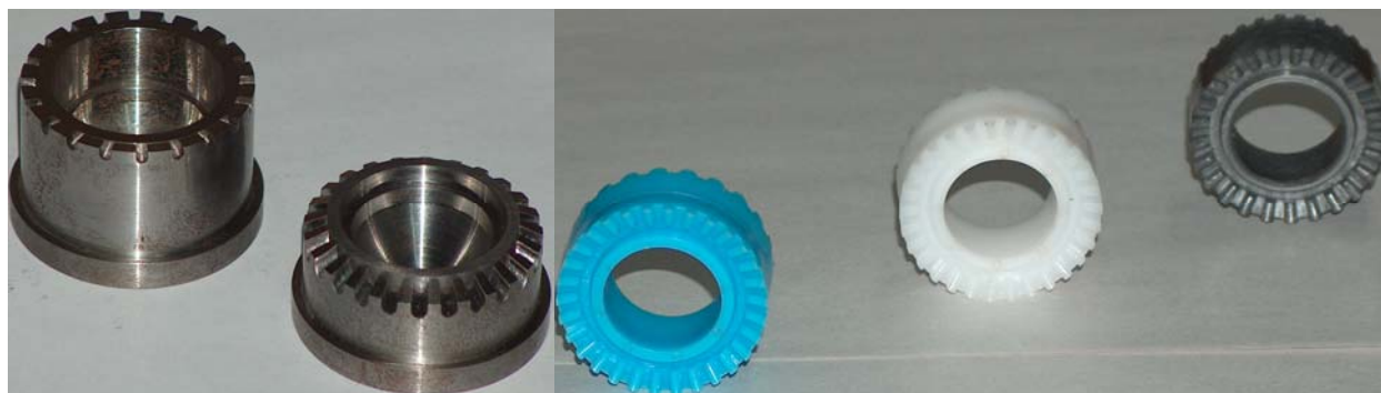
Figure 3. Set of moulds from the hollow mould.
