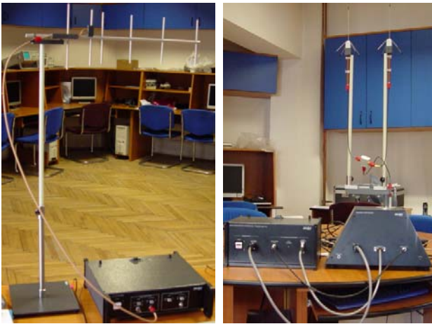
Fig. 4. Radio Frequency Generator – left and Antenna Positioner connected to Data Acquisition Interface – right.
