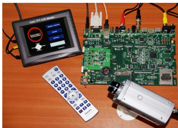
Figure 2. The DVEVM 6446 development platform
