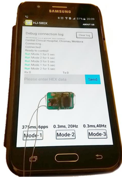
Fig.4 Wireless charged device with Bluetooth control.
