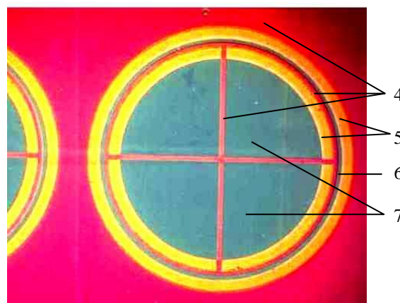
Figure 4. The circular photodiode-quadrant.
