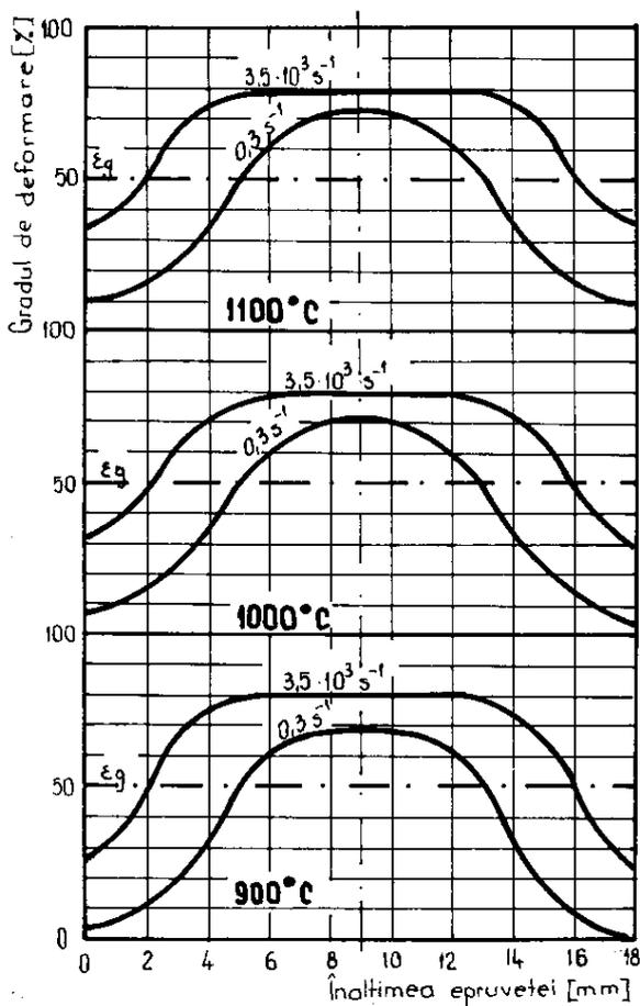
**Figure 3.** The dependency of deformation degree  $\varepsilon_g$  on the height of the specimen ( $h$ ) for the OLC45 steel.
