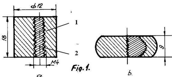
**Figure 1.** Cylindrical specimen  $\Phi 12 \times 18 \text{ mm}$ ; 2 – screw the M4; a) prior to upsetting; b) after the upsetting.
