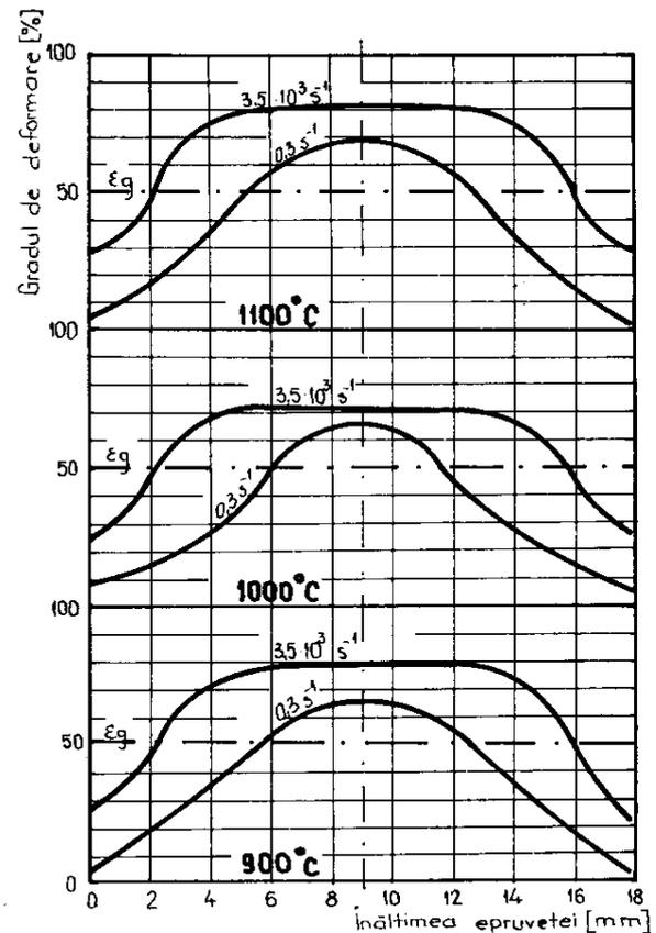
**Figure 2.** The dependency of deformation degree  $\varepsilon_g$  on the height of the specimen ( $h$ ) for the OLC15 steel.
