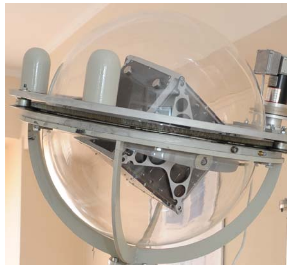
Figure 5. The Microsatellite mounted in the vacuumed planet gear carrier nest with spherical motion, NSTC, TUM.
