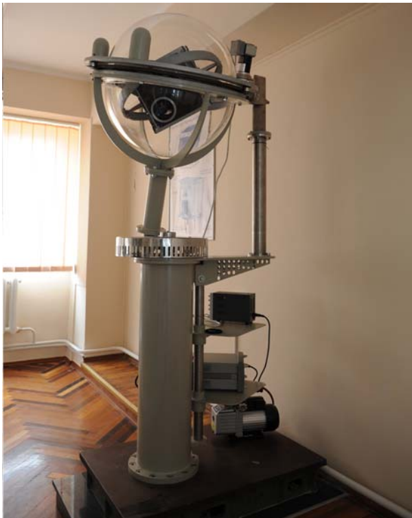
Figure 4. The simulator with the Microsatellite mounted in the external gyroscope, NSTC, TUM.
