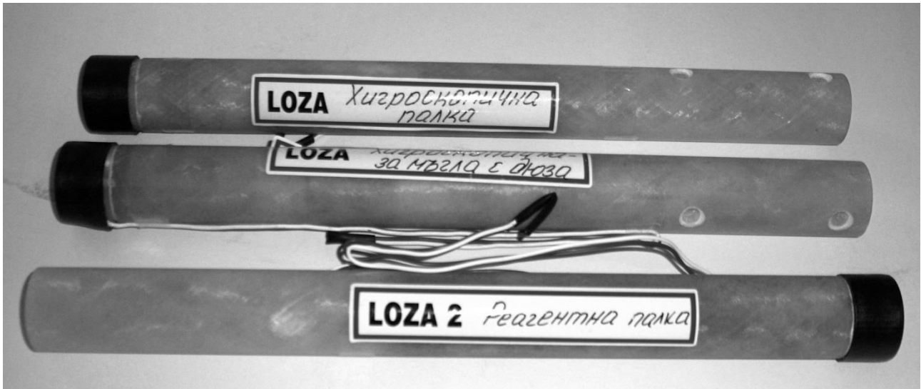
Fig.1. Samples of hygroscopic agents made in the form of reagent sticks.
