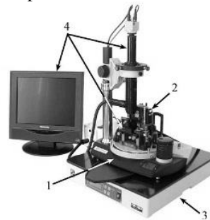
Fig. 2. NTEGRA Probe NanoLaboratory: a) 1 – base unit; 2 – measuring head; 3 – vibration isolation system; 4 – optical viewing system.
