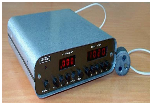
Fig. 4. The measurement device with the digit display of UV radiation with the intensity in limits of values 10^{-4} - 2 \cdot 10 mW/m 2 the spectral domains, nm: 280-400, 320-400, 320-360; the dose - 0 - 1.6 \cdot 10^5 J/m 2 .
