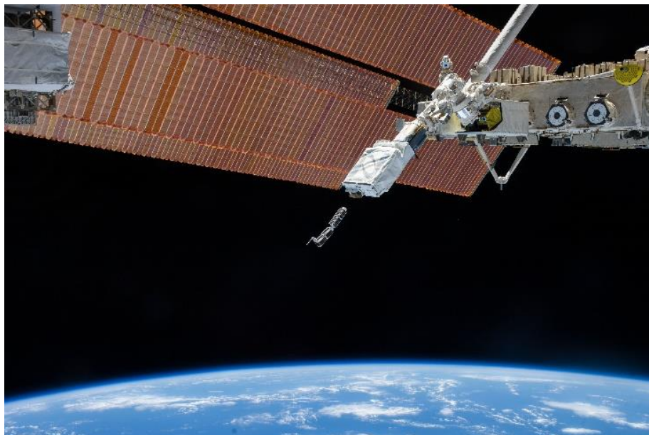
Figure 1: Nanosatellites deployment from JAXA Kibo Module.
