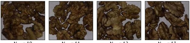
$N_{SCE} = 10$   $N_{SCE} = 11$   $N_{SCE} = 12$   $N_{SCE} = 13$ Figure 2. The external aspect of the walnuts kernels after extraction under the "step climb experience" conditions.
