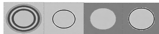
Fig. 1. The cross sections for different types of multilayer cylinder: 5-layer cylinder, the simplest type of nanotube, a cylindrical pore, metallized pore (different intensity of grey colour denotes different values of the dielectric constant).
