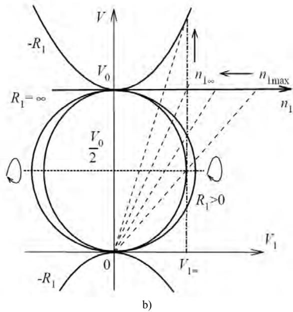
Fig.3 Bunch of circles for different  $R_1$  as  $V_{1=}$  (a) and bunch of curves at  $V_2 = 0$  and a point moving along lines  $V_{1=}$  (b)
