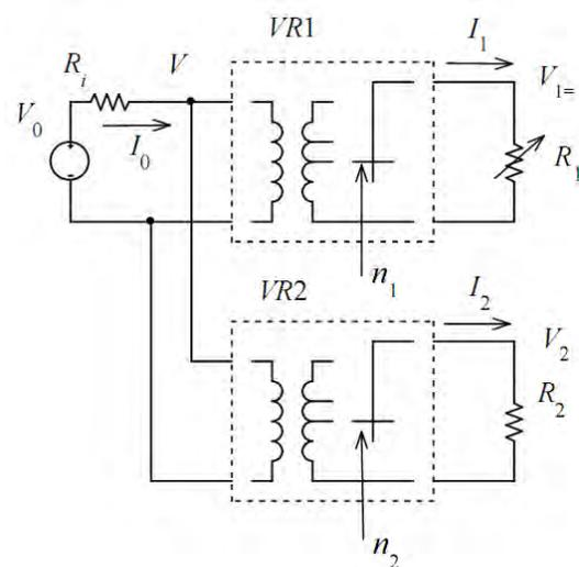
Fig.1 Power supply system with two regulators and loads
