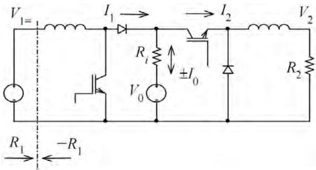
Fig.2 Power supply system with negative resistance  $-R_1$
