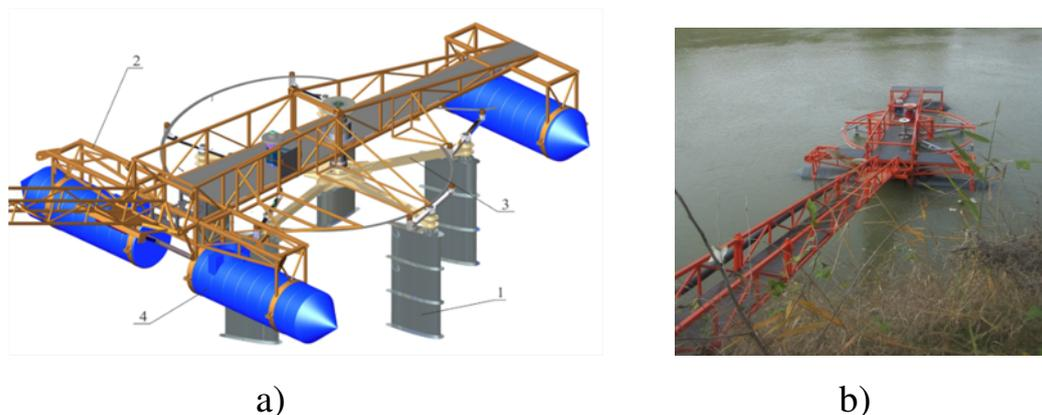
**Figure 2.** Flow micro hydropower plant with 5-blade tilting hydrodynamic rotor with cord length  $c = 800$  mm, submerged height  $h = 1600$  mm and screens for directing fluid flow (a). Industrial prototype of the micro hydropower plant installed on the test site on the Prut River (com. Stoienesti, Cantemir) (b).
