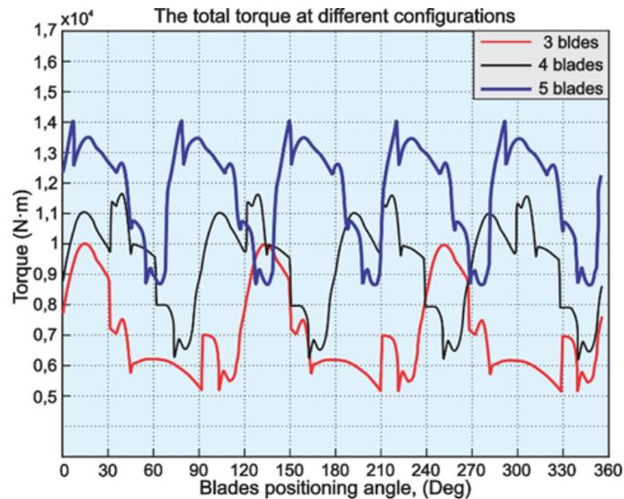
**Figure 1.** The total torque  $T_r, \Sigma$  developed at the rotor shaft with 3, 4 and 5 blades depending on the positioning angle.
