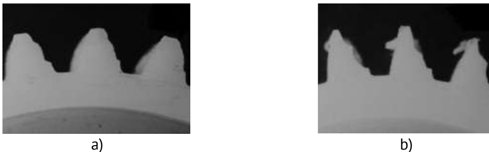
Figure 6. Wear of gear wheels made from: a) Nylon (PA6), b) Acetal (POM), module 3 mm, 30 teeth, [27].
