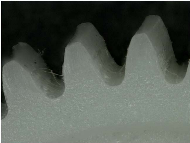
Figure 15. Wear damage on reinforced POM+ 10GF gear in pair with PA6+30GF after step test.
