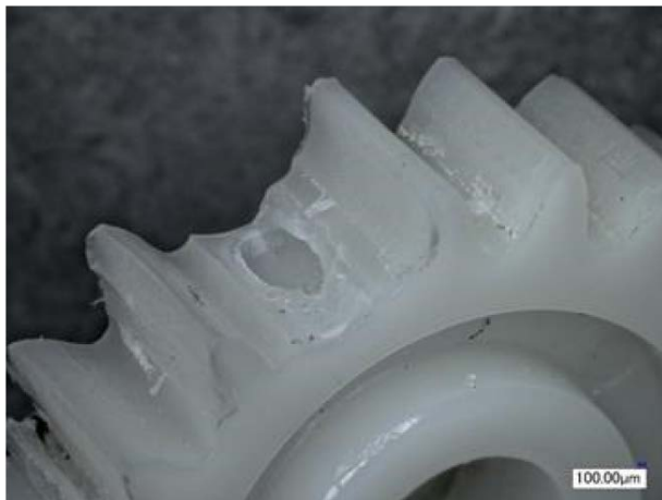
Figure 13. Sudden tooth fracture failure of POM gear is caused by fatigue and lunker created in the injection molding.
