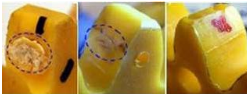
Figure 33. Wear at different pinions, [40].
