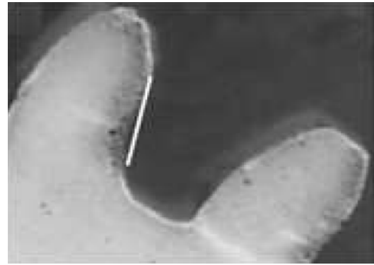
Figure 24. Reduction of the thickness of the polymeric tooth due to scraping of the opposite steel wheel, [35].
