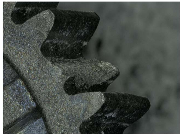
Figure 16. Fatigue failure mode of reinforced PPS+ 30CF/15 in pair with POM after 0.77 million load cycles at 1650 rpm and 0.5 Nm load level.
