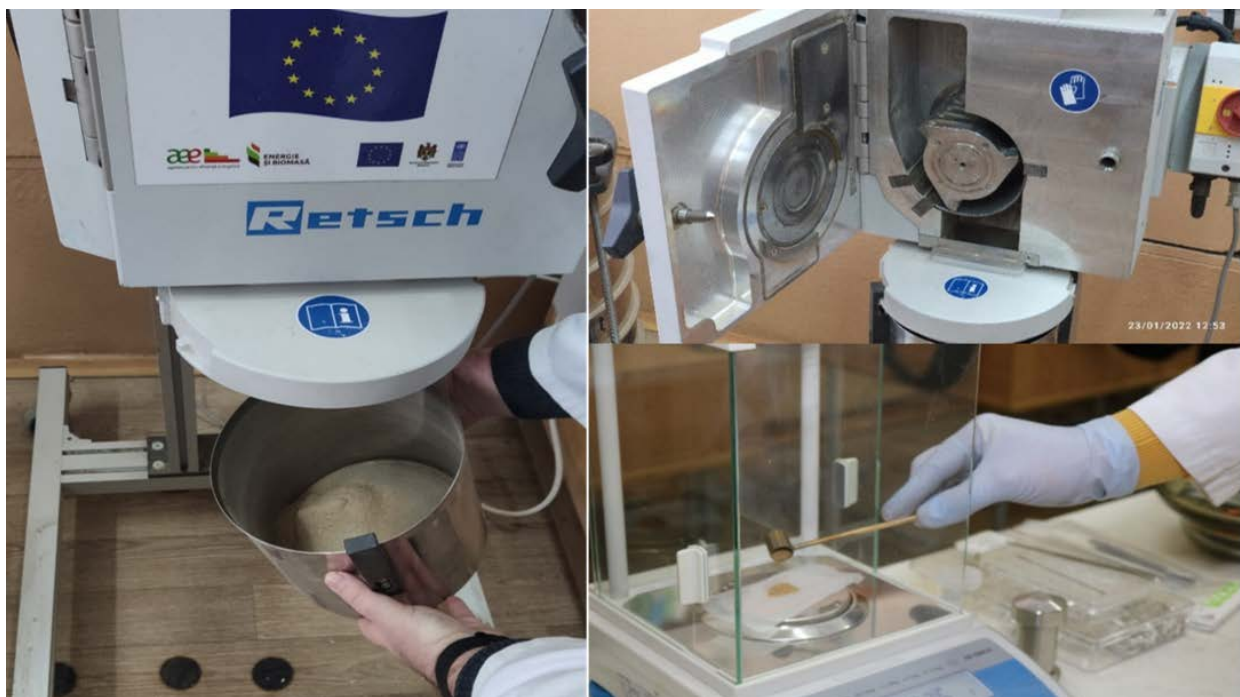
Figure 4. Pellet crushing and sample dosing by weighing.
