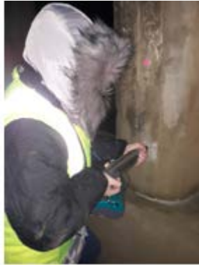
Figure 17. Determination of the compressive strength of concrete in pile columns.
