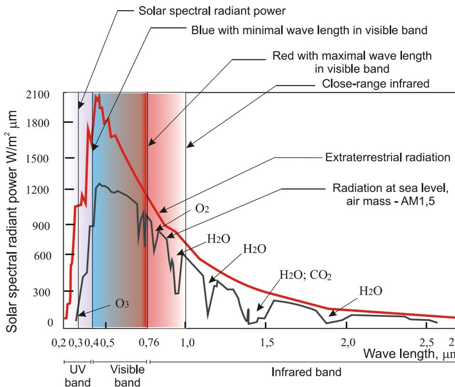
**Figure 6.** Spectral distribution of power flux (radiant) density.
