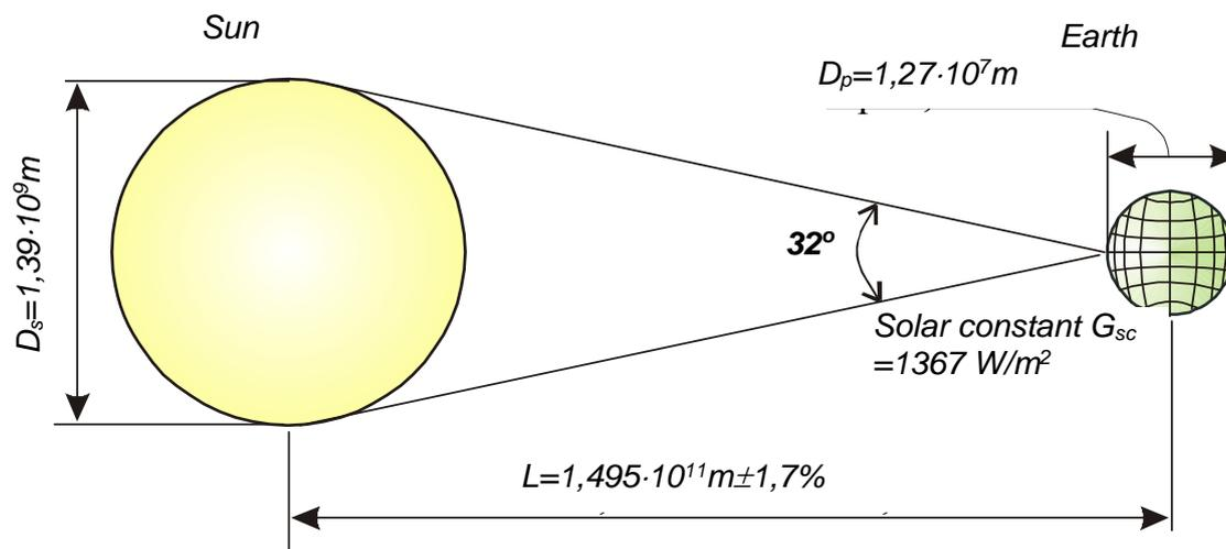
Figure 5. Geometry of the „sun-earth” system.
