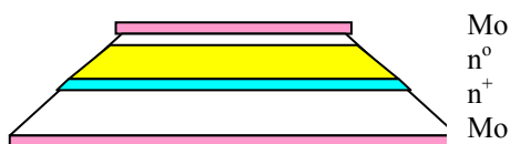
Fig.1 Recovery element with facet on p-n junction side (n 0 - base, Mo – molybdenum).
