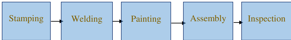
Figure 2. The flowchart of the manufacturing process [3]
