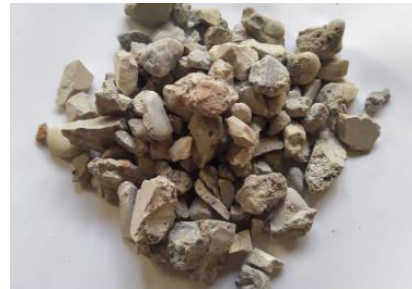
Figure 16. Secondary crushed stone with a heterogeneous composition (fractions 8-16 mm)
