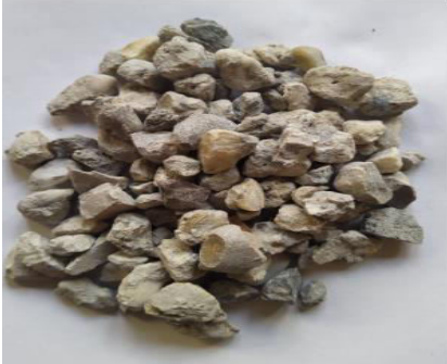
Figure 13. Secondary crushed stone and sand from concrete structures (fractions 0-5, 5-10, 10-20 mm)
