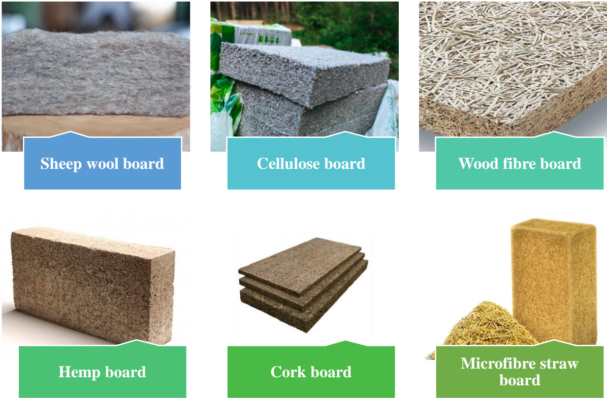
Figure 3. Types of sustainable insulation materials
