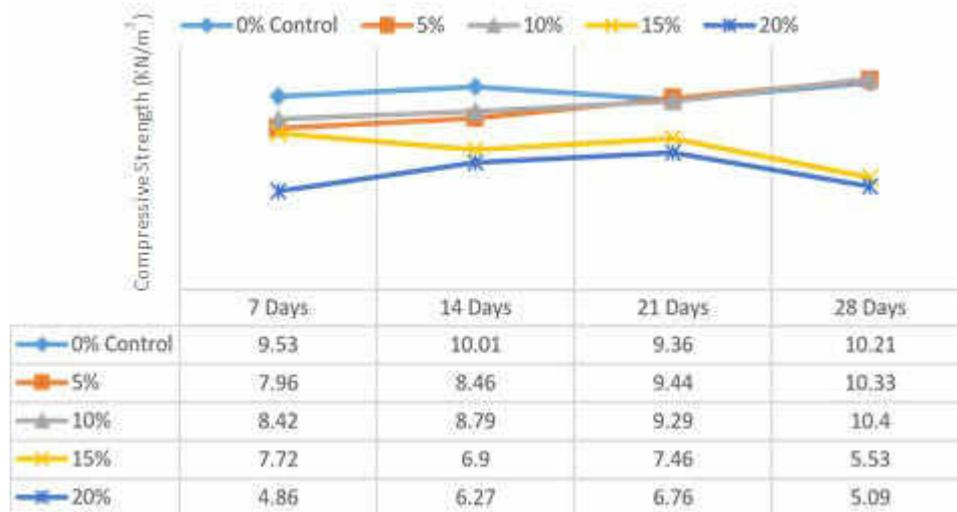
**Figure 4.** Compressive strength for % replacement of rice husk ash.
