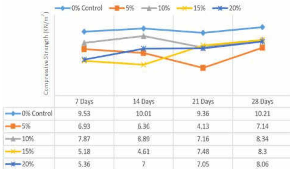
Figure 3. Compressive strength for % replacement with glass powder.
