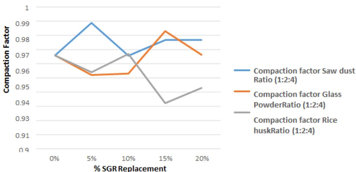
**Figure 1.** Compaction factor for saw dust ash, glass powder and rice husk ash.
