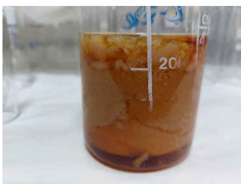
Figure 15. Formation of a calcium sediment with lactulose after electroactivation of lactose solution (4%) in the electrolyzer EDC-pilot, j=20 \text{ mA/cm}^2 .
