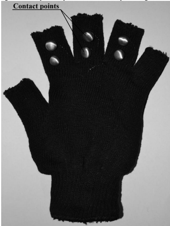
Figure 1. View of the glove from the side of flat of the hand. Here are situated contacts points which permits creating input signals for microcontroller which translates them into letters/words/phrases and send them wireless to desired device.
