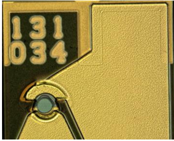
Fig. 5. Picture of the VCSEL chip with electroplated contact pads
