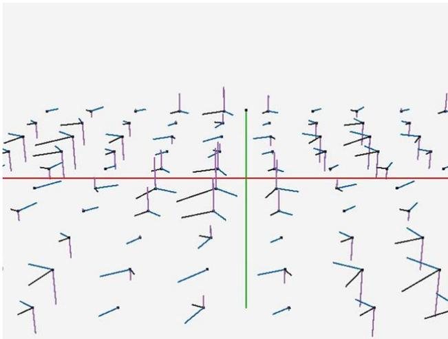
Fig. 2. It is illustrated wave-like light energy transfer in 2D field resulting from superposition of plane orthogonally polarized waves of equal amplitudes with the interference angle  $90^\circ$ . Energy transfer takes place along the bisectrix of the propagation directions of two waves at the incidence plane: the distribution of Poynting vector is presented in black color, of vector  $\vec{E}$  in blue and  $\vec{H}$  in violet.
