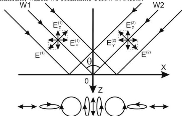
Fig. 1a. Superposition of plane waves of equal amplitudes linearly polarized at the incidence plane, with the interference angle  $90^\circ$ . Periodical spatial polarization modulation takes place at the incidence plane.
