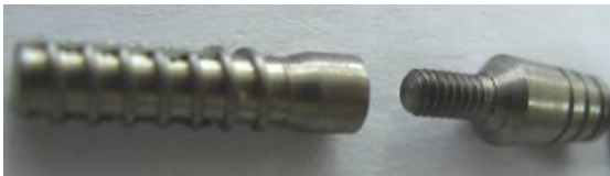
Fig. 2: Tapping component and abutment
