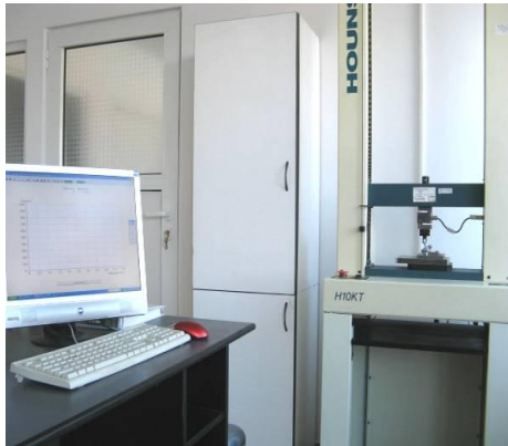
a) Static testing machine Hounsfield H10KT
