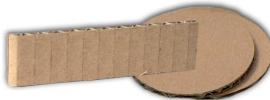
Fig 2 Samples of corrugated paperboard for ECT and FCT testing
