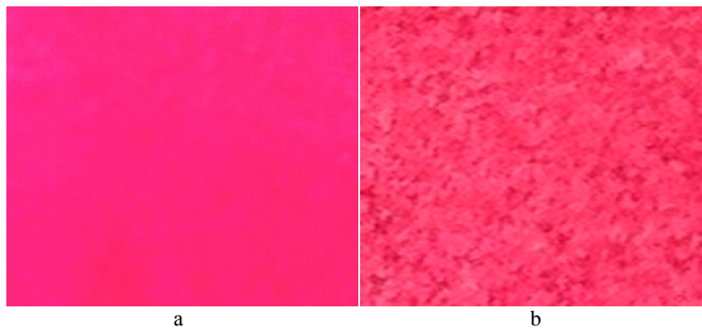
Fig. 4. Color paste (1:1) before drying (a), after drying (b)
