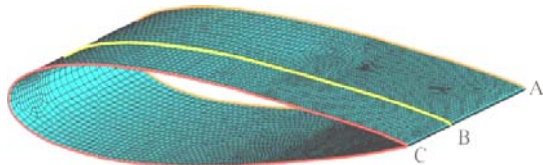
Figure 17. Discretization of the blade cover with Solsh190 finite elements.
