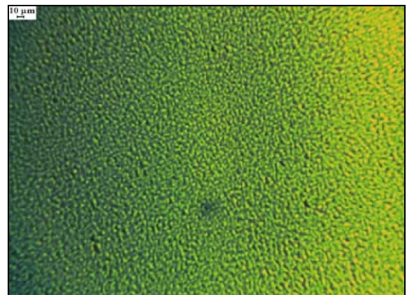
Fig. 1. Oxide layer image on GaAs plate on MM-500T microscope.
