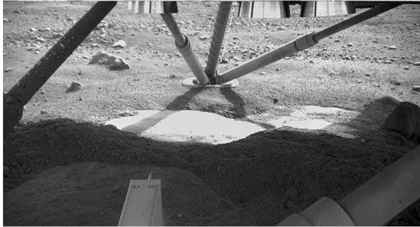
Figure 2. View underneath lander towards south foot pad, showing patchy exposures of a bright surface, possibly ice (Source: NASA)
